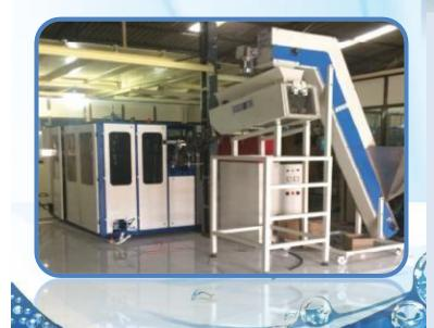
FULLY AUTOMATIC PET STRETCH BLOW MOULDING MACHINE. (BOTTLES)
